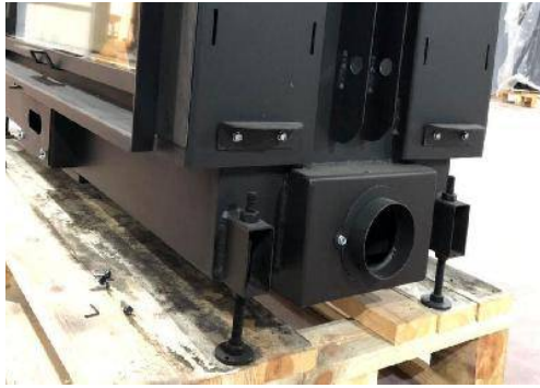
air supply pipe from outside (fresh air)
